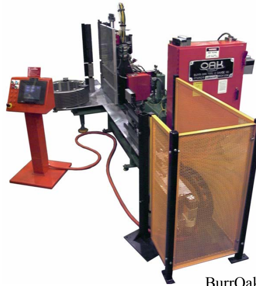
Figure 1—2: Burr Oak’s current coil forming machine
